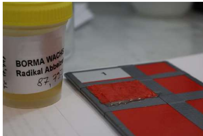
Photo 20: Testing of diferent chemical stripping methods
