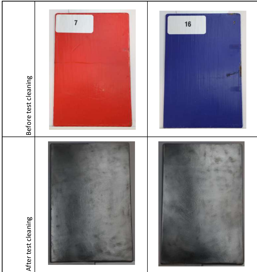
Photo 18: Test plates before and after the cleaning with rotating composite brushes
