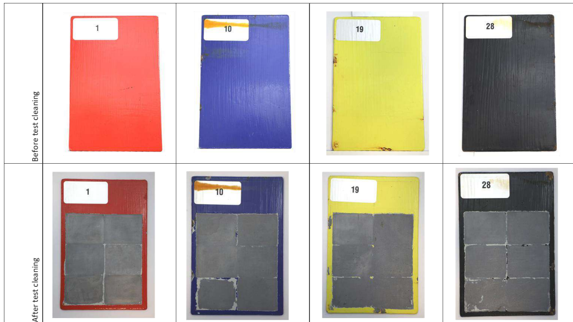
Photo 11: Test plates before and after the initial cleaning using 6 chemical stripping products
