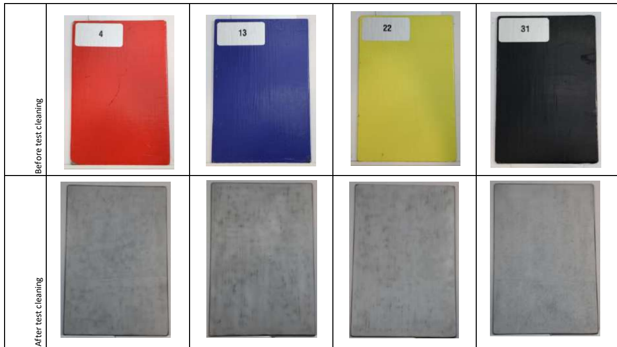
Photo 15: Test plates before and after the sandblasting with glass beads
