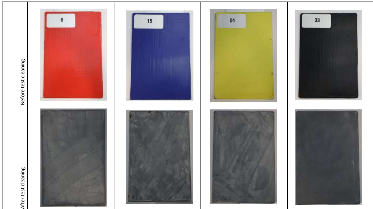
Photo 17: Test plates before and after cleaning with heatgun
