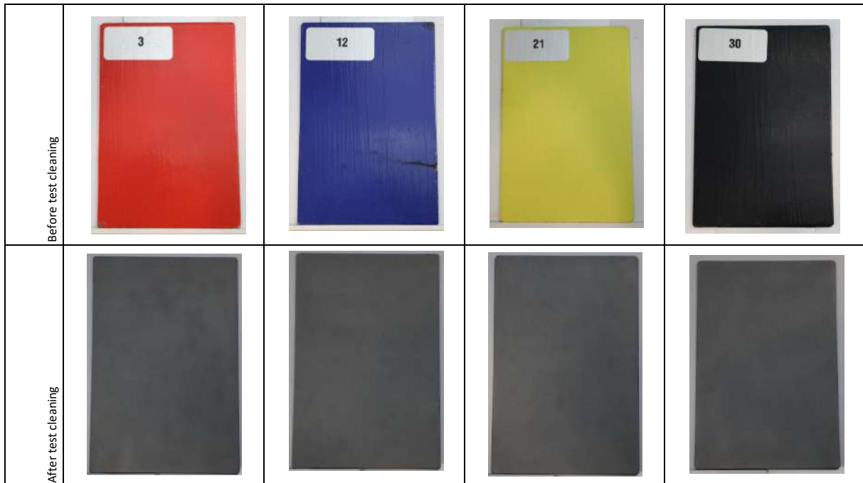
Photo 13: Test plates before and after the sandblasting with aluminium oxide
