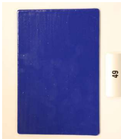
Photo 8: test plate before exposure in the salt spray chamber
