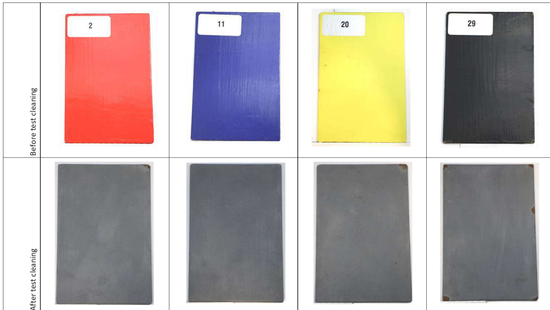
Photo 12: Test plates before and after the cleaning using the selected chemical stripping product
