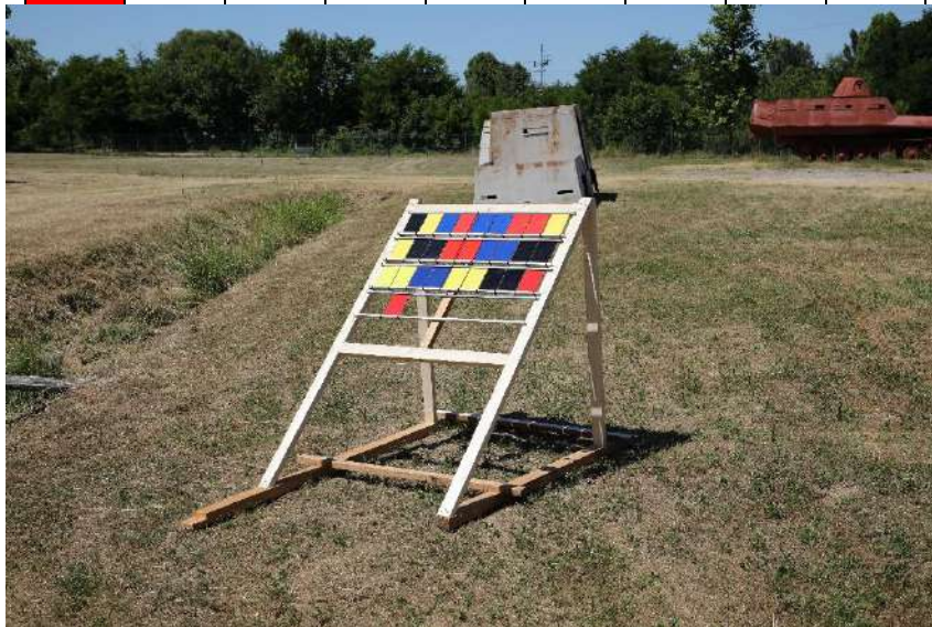
Photo 6: Outdoor exposure rack on the site of exposure inside the „Barutana“ complex in neighbourhood Caprag, Sisak
