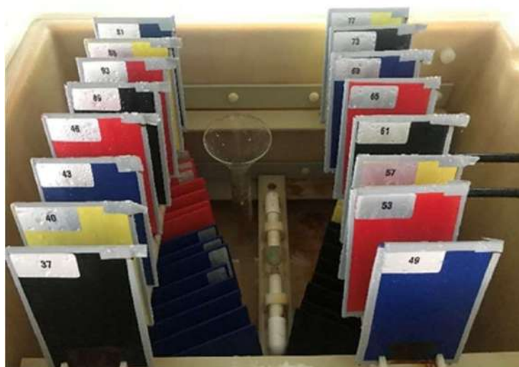
Photo 10: test plates during the ageing in the salt spray chamber
