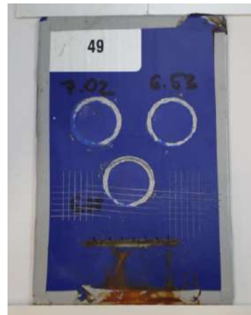
Photo 9: test plate after exposure in the salt spray chamber
