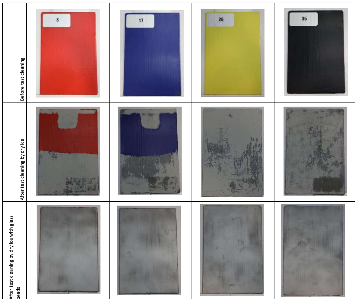
Photo 19: Teste plates before and after the cleaning using dry ice and dry ice with the adition of glass beads
