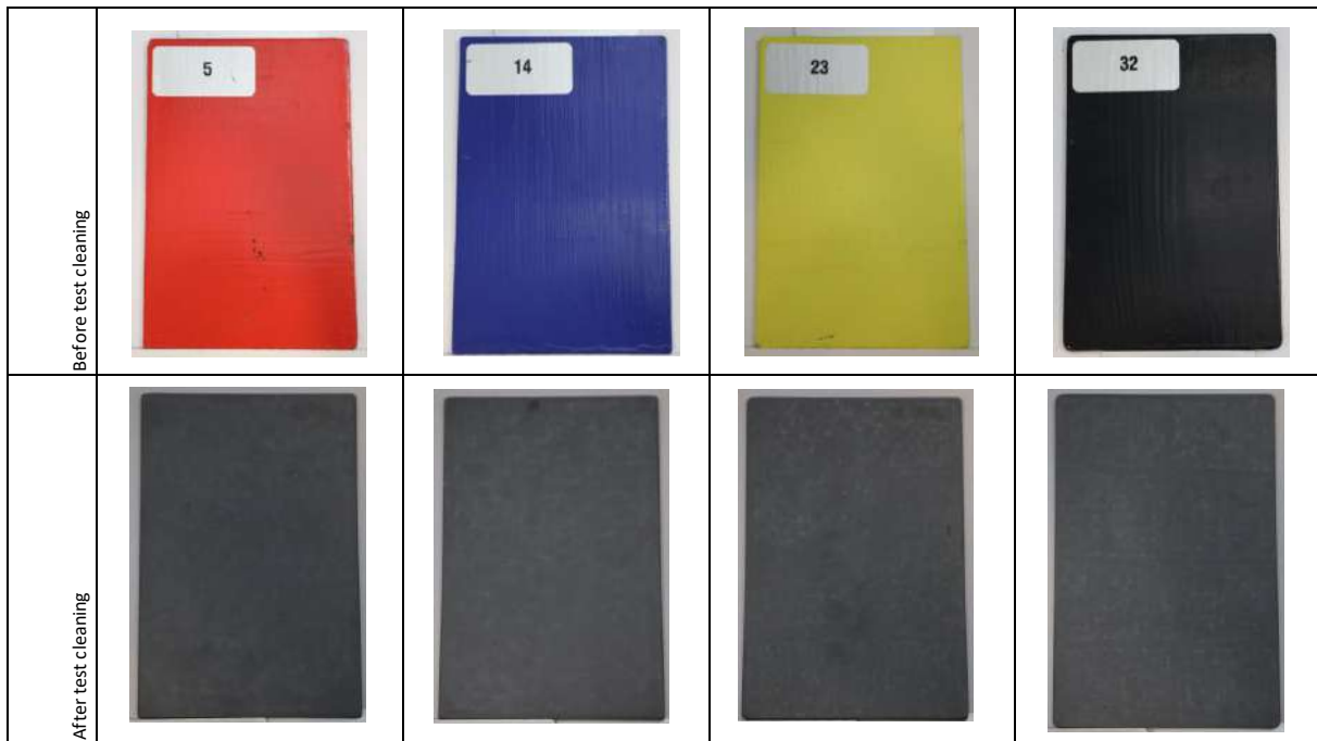
Photo 16: Test plates before and after sandblasting with nutshell granulate
