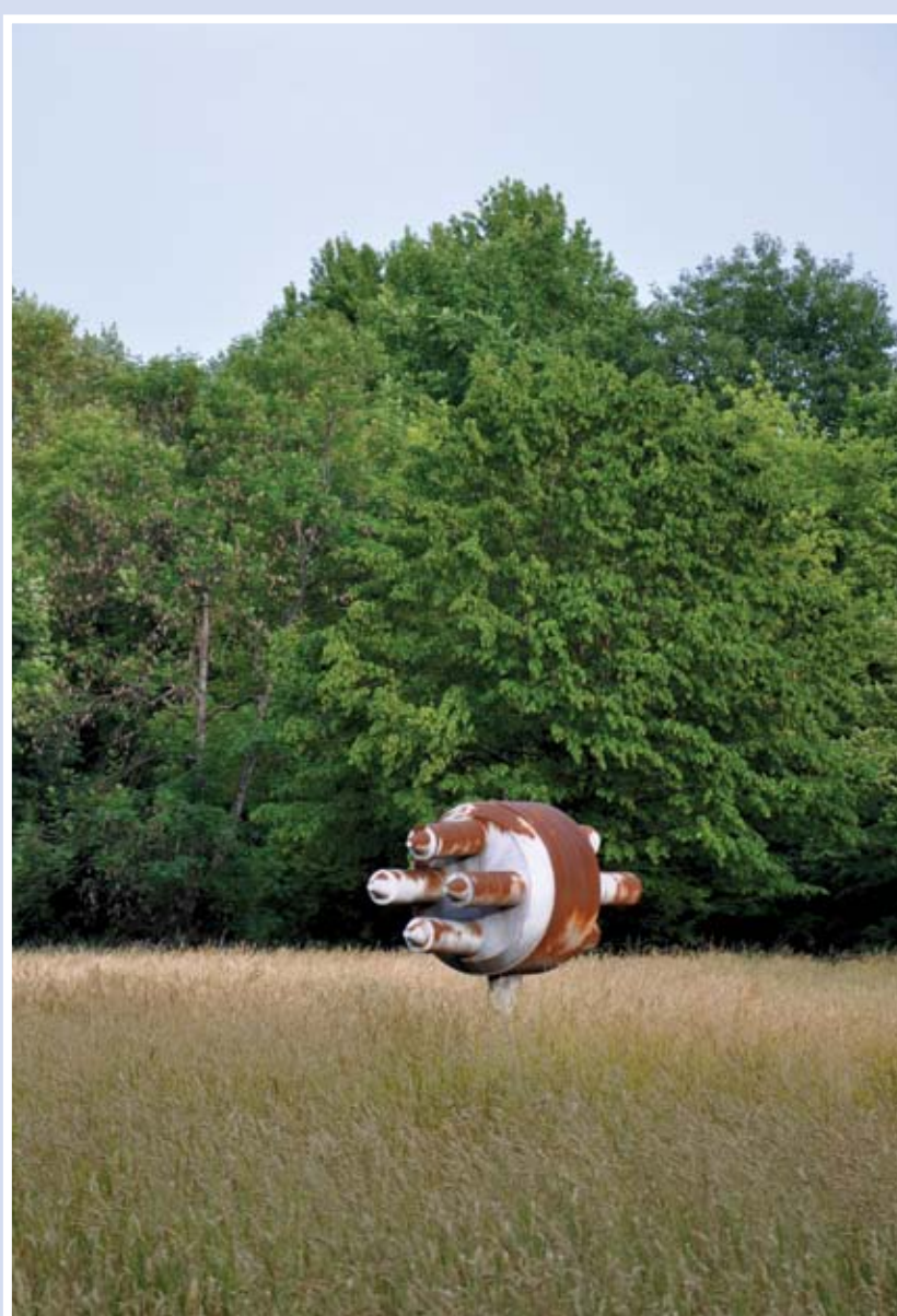
Figure 1 Josip Zeman's galvanized steel sculpture Dark Visions I of 1983 is severely corroded (photo: S. M. Sunara, May 2016)
