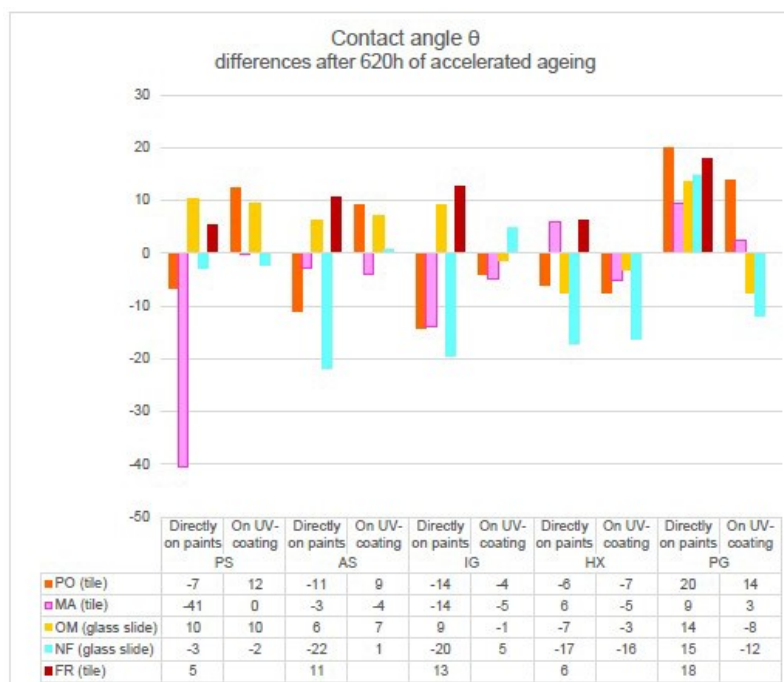
Figure 5 variation of contact angle values before and after the first step of the accelerated ageing
