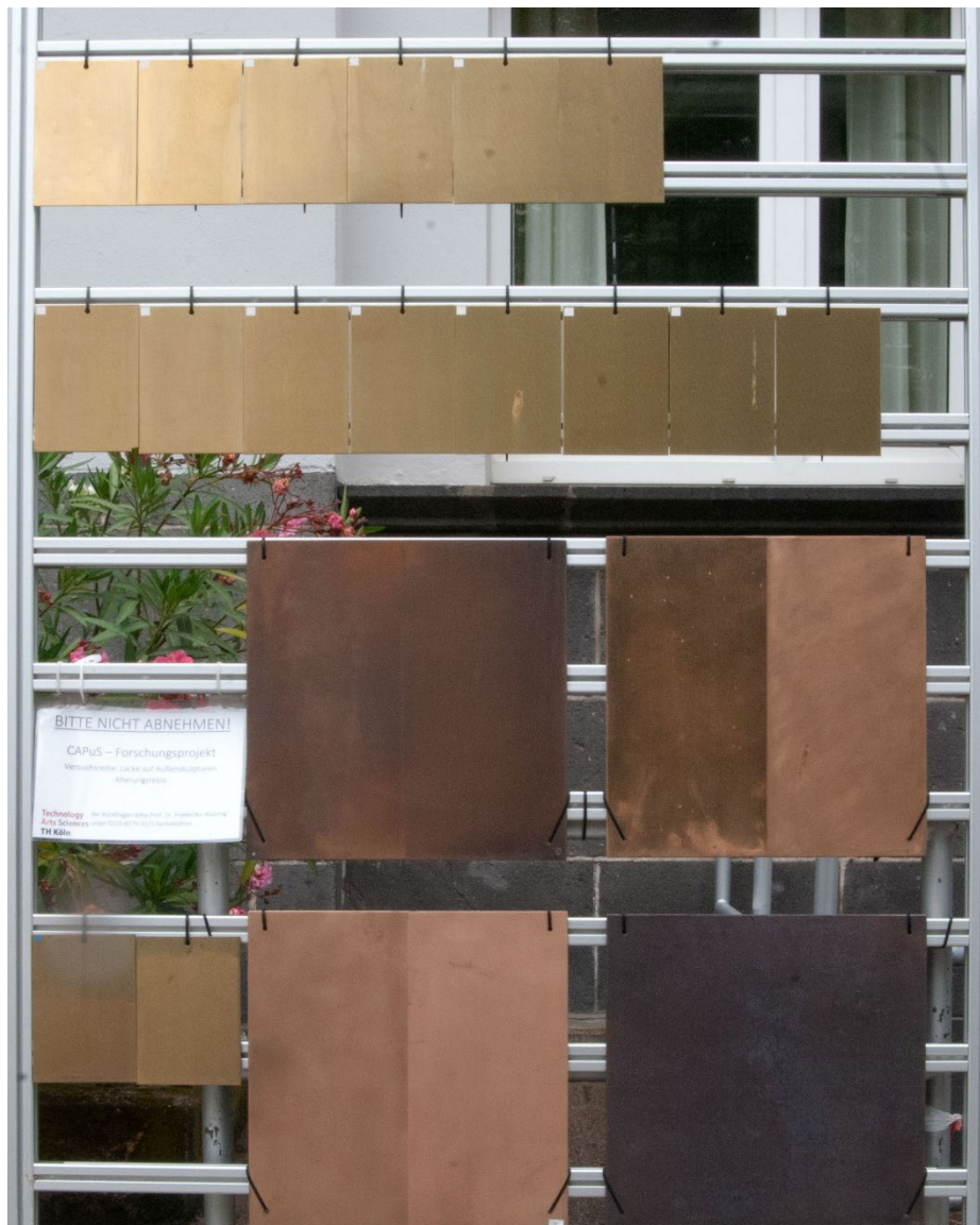
Figure 4: Weathering station with brass and bronze test plates
