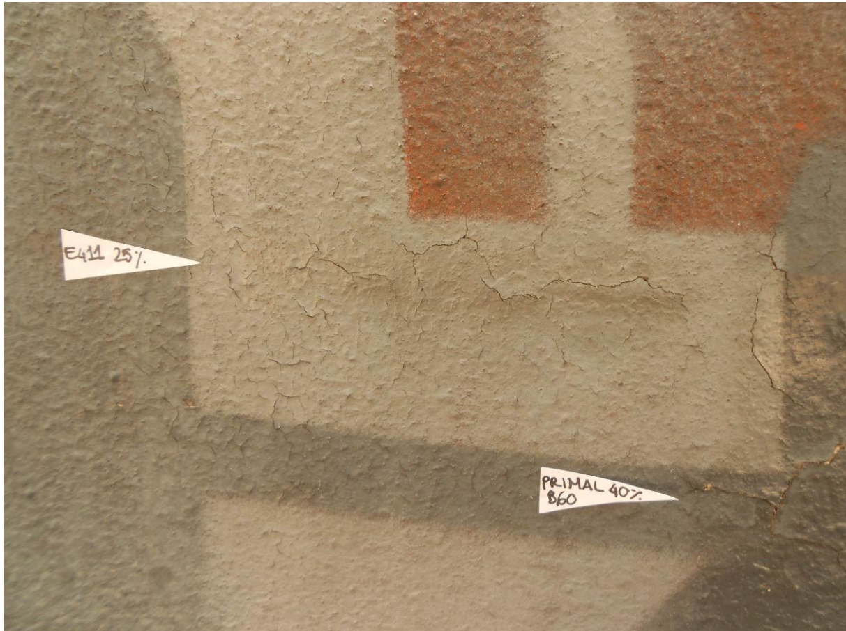
Fig. 1: Adhesion tests on site, showing the different behaviour of E411 and Primal B60A solutions.
