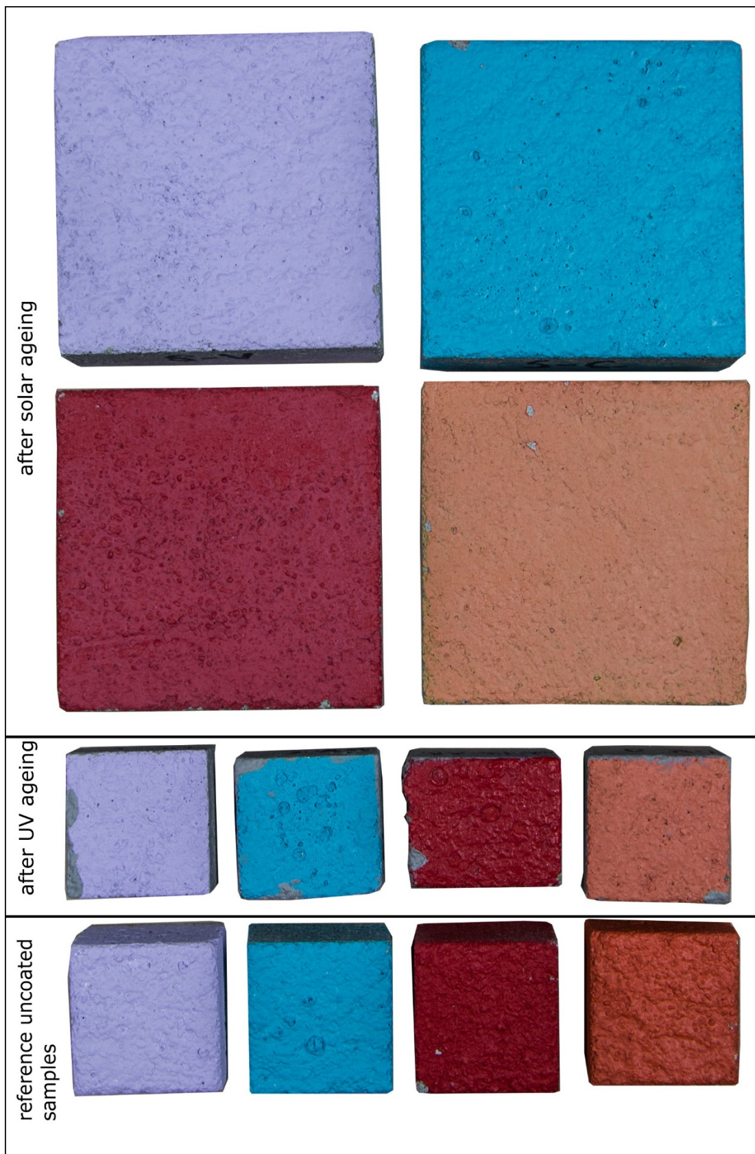
Figure 1 uncoated reference not aged samples (first row from the bottom), uncoated samples after UV aging (second row), uncoated samples after Solar aging (first row from the top)
