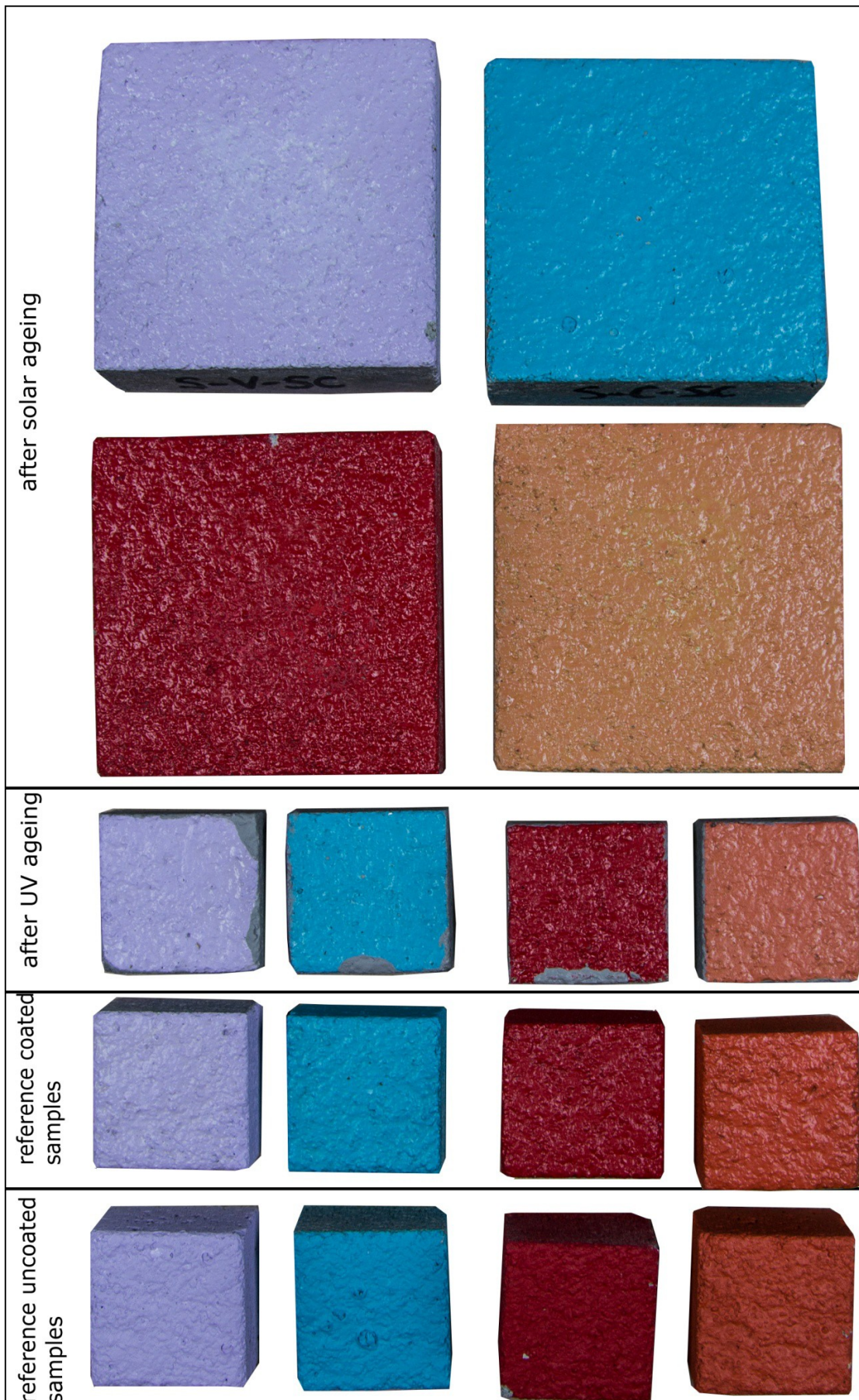
Figure 2 samples coated with ACPU-Clearlaquer and reference uncoated samples (bottom)
